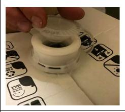
THE KEG HAS A VALVE THAT RELEASES THE CO2, IF PRESSED IN HIS SPECIAL ADAPTER. IT COULD CAUSE SOME NOISE.
